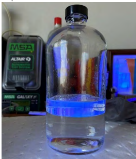
Figure 2: Jet A fuel floating on water illuminated by 365 nm UV flashlight. Photo courtesy of Bill Barth (ET).
